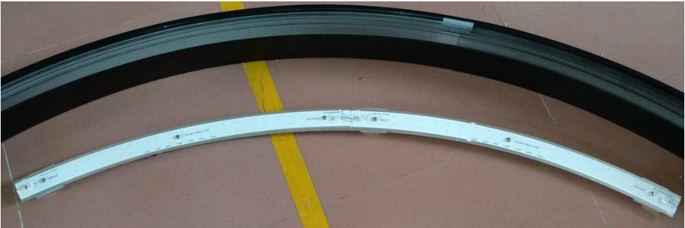
Reason 2: curved LED modules, mounted onto gear tray:
